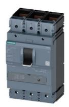
circuit breaker 3VA1 IEC frame 400 breaking capacity class M Icu=55kA @ 415V 3-pole, starter protection TM120M, AM, In=320A without overload protection short-circuit protection li=8...16 x In nut keeper kit
