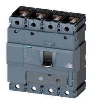
circuit breaker 3VA1 IEC frame 250 breaking capacity class S Icu=36kA @ 415V 4-pole, line protection TM240, ATAM, In=250A overload protection Ir=175A...250A short-circuit protection Ii=5...10 x In N conductor protection 100% nut keeper kit
