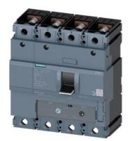
circuit breaker 3VA1 IEC frame 250 breaking capacity class S Icu=36kA @ 415V 4-pole, line protection TM240, ATAM, In=250A overload protection Ir=175A...250A short-circuit protection Ii=5...10 x In N conductor unprotected nut keeper kit
