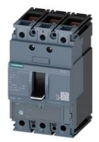
circuit breaker 3VA1 IEC frame 160 breaking capacity class M Icu=55kA @ 415V 3-pole, line protection TM220, ATFM, In=20A overload protection Ir=14A...20A short-circuit protection Ii=16 x In nut keeper kit
