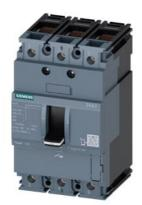
circuit breaker 3VA1 IEC frame 100 breaking capacity class N Icu=25kA @ 415V 3-pole, line protection TM210, FTFM, In=63A overload protection Ir=63A fixed short-circuit protection Ii=10 x In clamp connection
