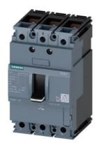
circuit breaker 3VA1 IEC frame 100 breaking capacity class B Icu=16kA @ 415V 3-pole, line protection TM210, FTFM, In=32A overload protection Ir=32A fixed short-circuit protection Ii=10 x In nut keeper kit
