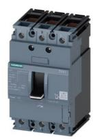
Circuit breaker 3VA1 IEC Frame 100 Switching capacity class N Icu=25 kA @ 415 V 3-pole, system protection TM210, FTFM, In=100 A Overload protection Ir=100 A non-adjustable short-circuit protection Ii = 10 x In Terminal connection
