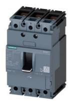
Circuit breaker 3VA1 IEC Frame 100 Switching capacity class N Icu=25 kA @ 415 V 3-pole, system protection TM210, FTFM, In=100 A Overload protection Ir=100 A non-adjustable short-circuit protection Ii = 10 x In Lug terminal
