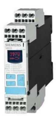
Digital monitoring relay Asymmetry 0-20% Phase sequence can be activated Phase failure 3 x 160 to 690 V 50 to 60 Hz AC Undervoltage 160-690 V Hysteresis 1-20 V ON and OFF delay 0-20 s 2 change-over contacts spring-type connection system
