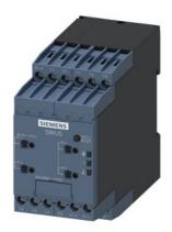
insulation monitoring relay for non-grounded (IT) networks up to 400 V AC, 15-400 Hz and up to 600 V DC measuring range 1-100 / 2-200 kOhm supply voltage 24-240 V AC/DC width 45 mm 1 + 1 or 2 changeover contacts screw terminal
