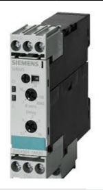
ANALOG MONITORING RELAY FILL LEVEL MONITORING RESISTANCE MONITORING FROM 2 TO 200 KOHM OVERSHOOT AND UNDERSHOOT AC/DC 24 TO 240V DC AND AC 50 TO 60 HZ 2-POINT OR 1-POINT CONTROL TRIPPING DELAYED 0.5 TO **10S 1 CHANGEOVER CONTACT SCREW TERMINAL REPLACEMENT PRODUCT F. 3UG3501**
