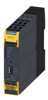
SIRIUS SAFETY RELAY BASIC UNIT ADVANCED SERIES WITH TIME DELAY 0.05-3S RELAY ENABLING CIRCUITS 2 INSTANTANEOUS NO CONTACTS 2 DELAYED NO CONTACTS US = 24 V DC SPRING-LOADED TERMINAL
