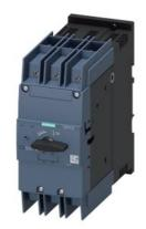
Circuit breaker size S3 for system protection with approval circuit breaker UL 489, CSA C22.2 No.5-02 A-release 40 A N-release 520 A screw terminal
