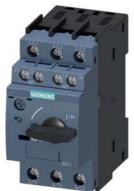
Circuit breaker size S0 for motor protection, CLASS 10 A-release 30...36 A N-release 432 A screw terminal Standard switching capacity with transverse auxiliary switches 1 NO+1 NC
