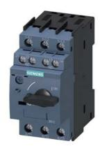
Circuit breaker size S00 for motor protection, CLASS 10 A-release 9...12 A N-release 163 A screw terminal Standard switching capacity with transverse auxiliary switches 1 NO+1 NC
