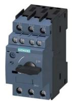
Circuit breaker size S00 for motor protection, CLASS 10 A-release 3.5...5 A N release 65 A screw terminal Standard switching capacity with transverse auxiliary switches 1 NO+1 NC
