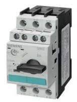
Circuit breaker size S0 for motor protection CLASS 10 A-release 7...10 A Short-circuit release 130 A Screw terminal Standard switching capacity with transverse auxiliary switch 1 NO+1 NC !!! Phased-out product !!! Successor is SIRIUS 3RV2 Preferred successor type is >>3RV2011-1JA15<<
