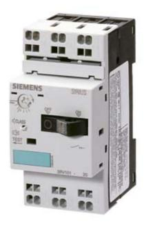
CIRCUIT-BREAKER, 3.5...5 A N-RELEASE 65 A, SIZE S00 MOTOR PROTECTION, CLASS 10, CAGE CLAMP CONNECTION STANDARD BREAKING CAPACITY
