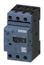
Circuit breaker size S00 for motor protection, CLASS 10 A-release 0.9...1.25 A N-release 16 A Screw terminal Standard switching capacity
