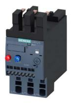
Overload relay 11...16 A Thermal For motor protection Size S0, Class 10 Contactor mounting Main circuit: Spring-type terminal Auxiliary circuit: spring-type terminal Manual-Automatic-Reset
