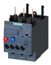
Overload relay 2.2...3.2 A Thermal For motor protection Size S0, Class 10 Contactor mounting Main circuit: Screw Auxiliary circuit: Screw Manual-Automatic-Reset
