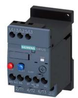
Overload relay 2.8...4.0 A Thermal For motor protection Size S00, Class 10 Standalone installation Main circuit: Screw Auxiliary circuit: Screw Manual-Automatic-Reset
