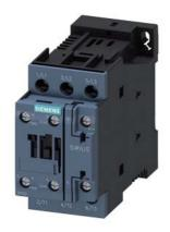
Power contactor, AC-3 32 A, 15 kW / 400 V 1 NO + 1 NC, 24 V DC 3-pole, size S0 screw terminals
