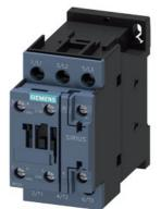
power contactor, AC-3e/AC-3, 25 A, 11 kW / 400 V, 3-pole, 230 V AC, 50 Hz, auxiliary contacts: 1 NO + 1 NC, screw terminal, size: S0
