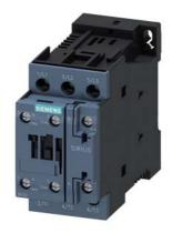
power contactor, AC-3 9 A, 4 kW / 400 V 1 NO + 1 NC, 24 V DC 3-pole, Size S0 screw terminal
