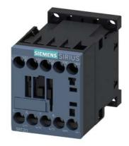
power contactor, AC-3e/AC-3, 7 A, 3 kW / 400 V, 3-pole, 24 V DC, with integrated diode, auxiliary contacts: 1 NC, screw terminal, size: S00
