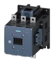
Power contactor, AC-3 400 A, 200 kW / 400 V AC (50-60 Hz) / DC operation 23-26 V UC Auxiliary contacts 2 NO + 2 NC 3-pole, Size S12 Busbar connections Drive: conventional screw terminal
