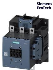
power contactor, AC-3e/AC-3 150 A, 75 kW / 400 V AC (50-60 Hz) / DC Uc: 110-127 V 3-pole, auxiliary contacts 2 NO + 2 NC drive: conventional main circuit: busbar control and auxiliary circuit: screw terminal
