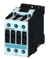
Power contactor, AC-3 12 A, 5.5 kW / 400 V 230 V AC, 50 Hz 3-pole, Size S0 Screw terminal III Phased-out product III Successor is SIRIUS 3RT2 Preferred successor type is >>3RT2024-1AP00<<
