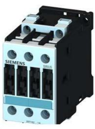
CONTACTOR, AC-3 4KW/400V, AC 230V 50HZ, 3-POLE, SIZE S0, SCREW CONNECTION
